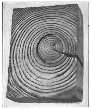
Fig. 44.—Cross section of timber showing several kinds of defects.
